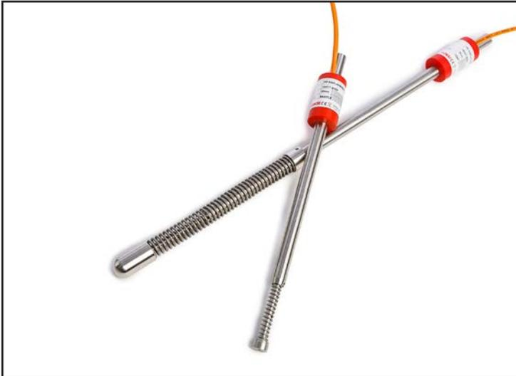
Geosense® VWDT-6000 series of spring-loaded vibrating wire displacement transducers which cover displacement ranges up to 75mm and are fully waterproof to a minimum of IP68 (16 bar external pressure). They can be incorporated into many displacement products such as crack joint meters, convergence meters, soil extensometers and displacement meters.
