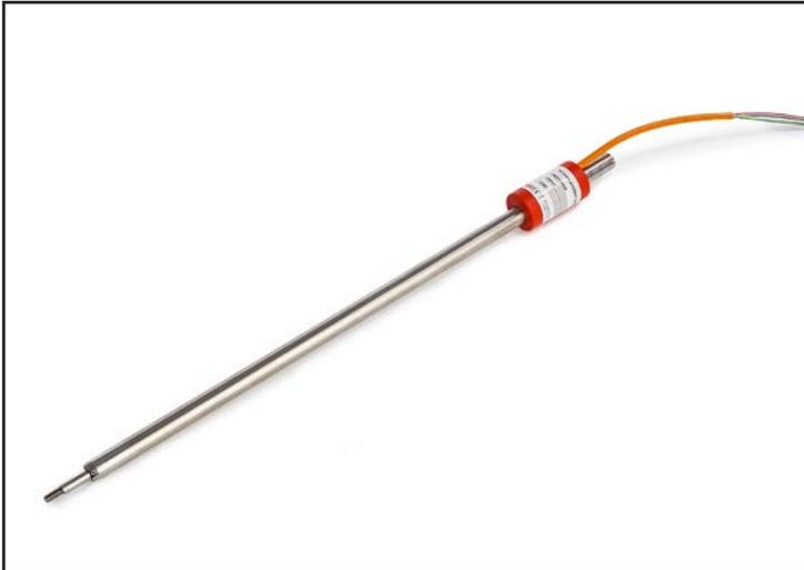
Geosense® VWDT-5000 series of vibrating wire displacement transducers cover displacement ranges up to 300mm and are fully waterproof to a minimum of IP68 (16 bar external pressure). They can be incorporated into many displacement products such as crack and joint meters, convergence meters, soil extensometers and displacement meters.
