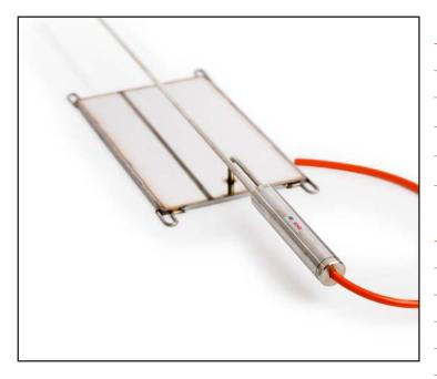
Geosense® NPC-3000 Series NATM Pressure cells are designed to monitor stress of shotcrete in the construction of tunnels, particularly those using the New Austrian Tunnel Method and other underground works. Monitoring of the radial and tangential stresses within shotcrete linings is vital to its success.
