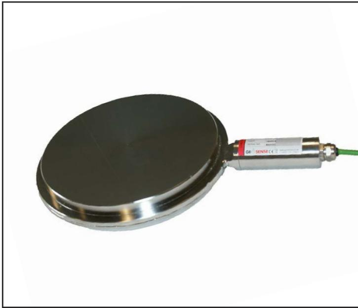
This consists of a sensitive pressure pad formed by joining two stiff steel discs at their periphery. The void inside the cell is filled with de-aired fluid. When load is applied to the cell the pressure of the inside liquid changes. The changes in pressure correspond directly to the load applied.
