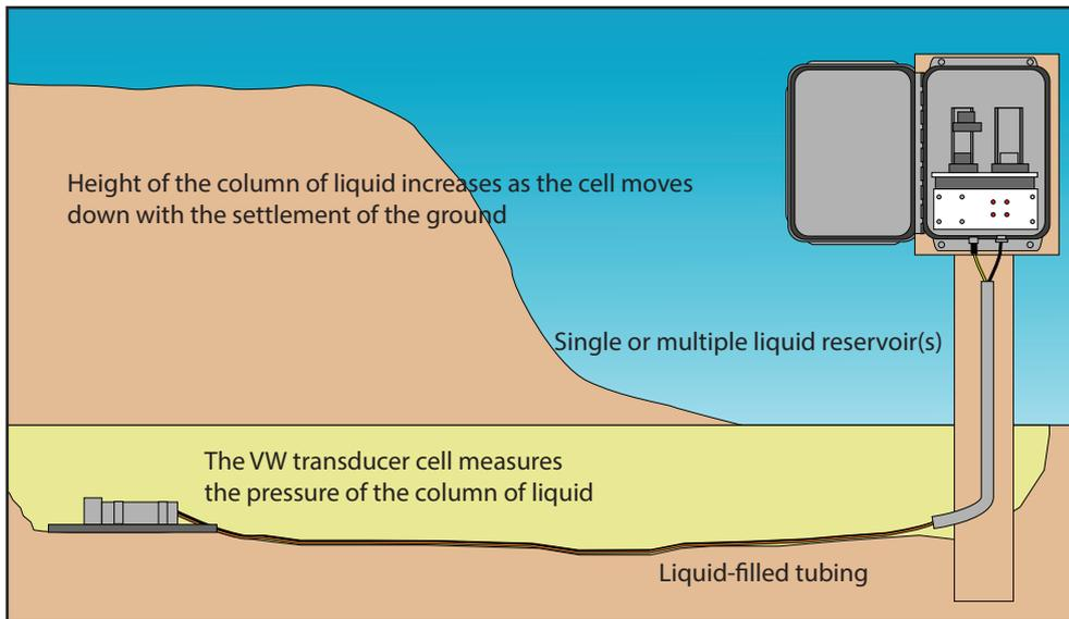
The pressure sensor transducer uses a pressure sensitive diaphragm with a vibrating wire element attached to it which is mounted inside an evacuated and hermetically sealed housing. Various housings are available to suit application.
