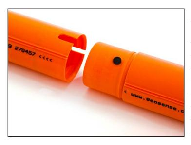
Geosense® QJ Inclinometer Casing is a quick connecting casing, precision extruded from ABS, with four precise keyways formed at 90 degrees which allow accurate installation of portable and in-place inclinometers.
