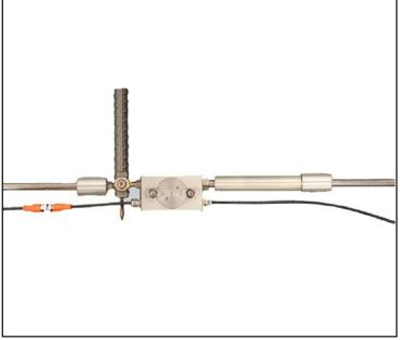
The Tunnel Profile Monitoring System is a series of linked rods fixed to the tunnel wall to monitor deformation. A data logging system and related software is available to provide near real time displacement and generate a graphical representation of the tunnel performance.
