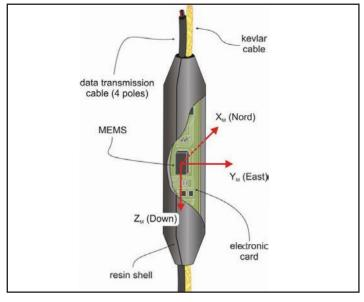
The Geosense® TiltArray™ can be used to monitor the magnitude and direction of lateral deformation vertically, and vertical deformation horizontally.
