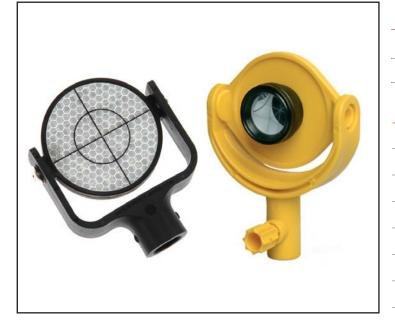
Geosense<sup>®</sup> Model GSRT-2 is a 2-dimensional reflective Bireflex target used primarily for tunnel convergence monitoring. It has reflectors on both sides and is mounted on a universal joint so it can be orientated in any direction required.
