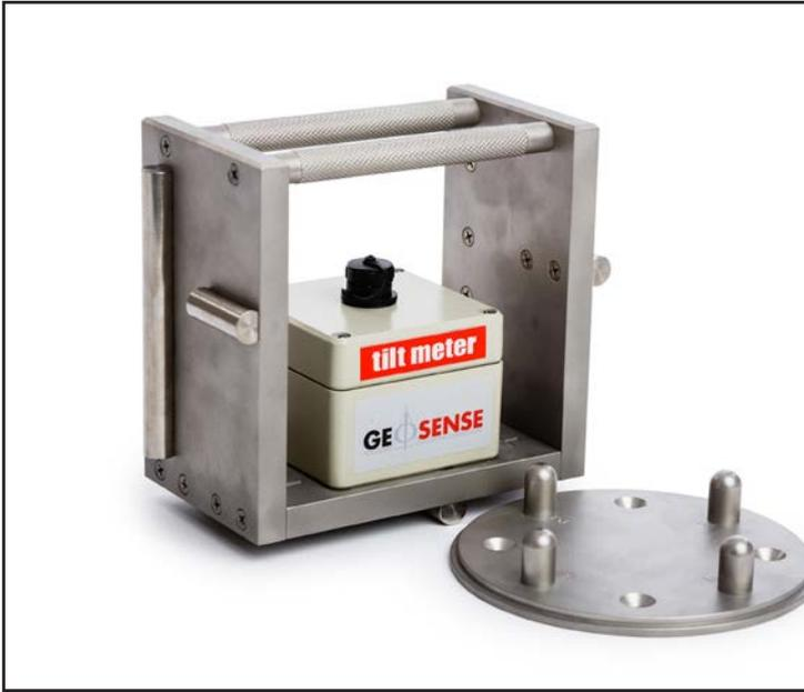
Portable MEMS Tilt Meters use a MEMS inclinometer to measure tilt in either one or two axial planes, perpendicular to the surface of the base plate. Depending on the model, the output is an analog DC signal or digital output and is directly proportional to the sine of angle of tilt.
