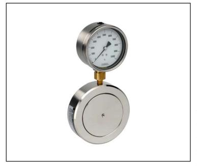
The Geosense® HLC-6050 series of Hydraulic Load Cells consist of a sensitive pressure pad formed by joining two stiff steel discs at their periphery. The void inside the cell is filled with de-aired fluid. When load is applied to the cell the pressure of the inside liquid changes. The changes in pressure correspond directly to the load applied.
