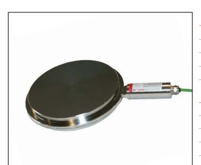
This consists of a sensitive pressure pad formed by joining two stiff steel discs at their periphery. The void inside the cell is filled with de-aired fluid. When load is applied to the cell the pressure of the inside liquid changes. The changes in pressure correspond directly to the load applied.
