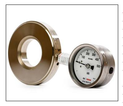
The Geosense® HLC-6000 series Hydraulic Anchor Load Cells consist of a sensitive pressure pad formed by joining two stiff steel discs at their periphery. The void inside the cell is filled with de-aired fluid. When load is applied to the cell the pressure of the inside liquid changes. The changes in pressure correspond directly to the load applied.
