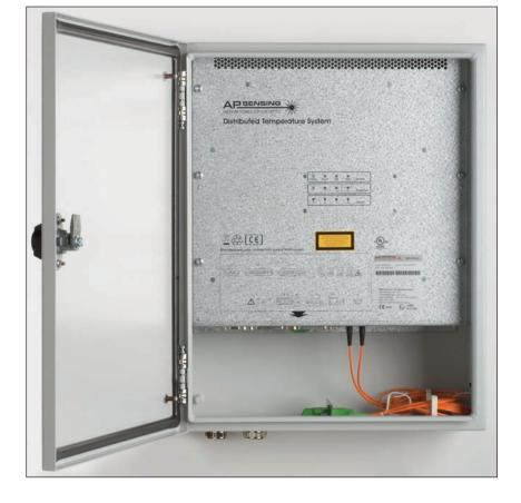
The Geosense<sup>®</sup> GEO-001I interrogator utilises Raman scattering to determine the change in temperature along a single optical fibre. The exact location of the measurement is determined from a precise time measurement.
