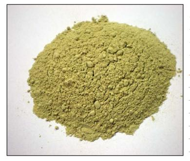
Grout Mix is a pre-blended powder mixture of Ordinary Portland Cement (CEM 1) and a premium grade high quality sodium carbonate activated Bentonite powder in a ratio of 2:1.
